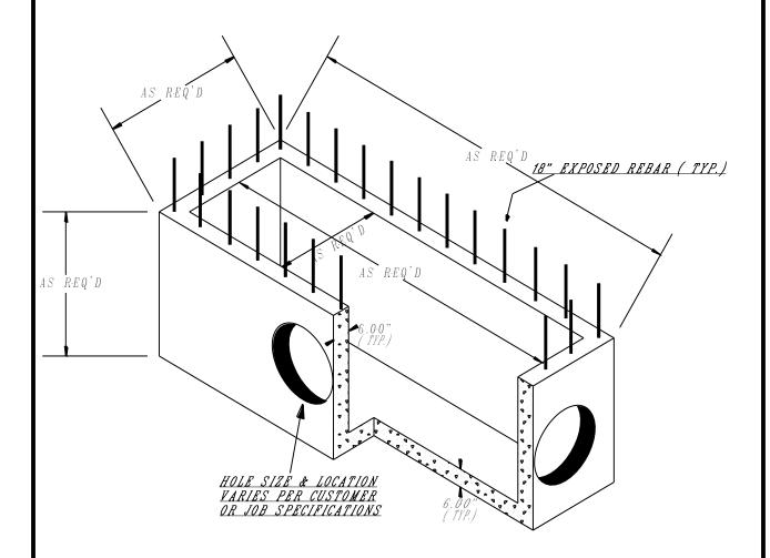
ALL CURB INLETS LEFT APPROX. 18" SHORT W/ 18" EXPOSED REBAR AT TOP. TOPS AND REST OF WALLS TO BE POURED IN THE FIELD.
